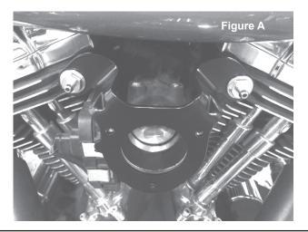
■ Install welded backing plate (11) using the 3 1/4-20 socket cap screws (2) into corresponding throttle body threaded holes as shown in FIG B. Torque 1/4-20 socket cap screws to 40-60 In-lbs.
